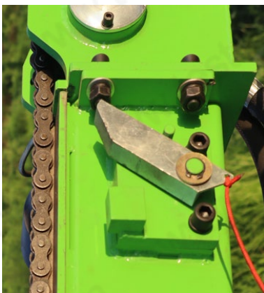
Figure 2: To release the securing device, the rope of the securing pawl is pulled and the impact unit is moved past it
