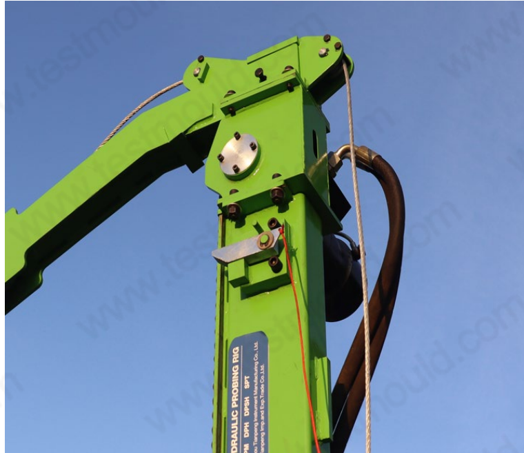
Figure 1: Impact device is properly placed on safety claws
